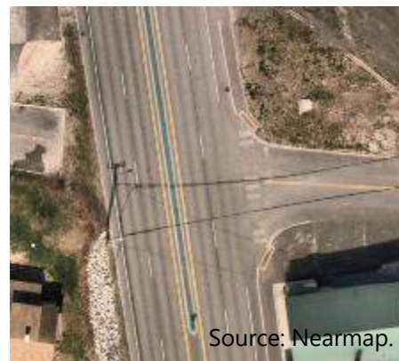
Figure 18: Install thermoplastic tape or inlay to reduce fading at crosswalk on Oak Hill Road
