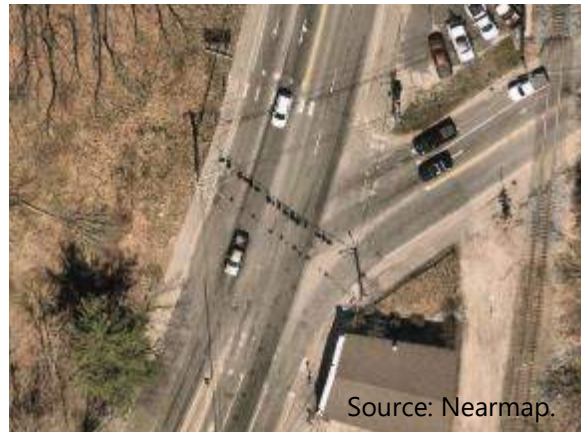
Figure 66: Install reflective thermoplastic tape or inlay at Washington Street North/Minot Avenue at High Street crossings
