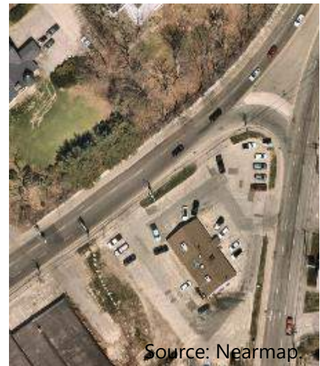
Figure 48: Example of need to consolidate driveways at commercial land uses
